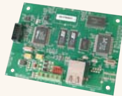
E080-2 Galaxy Ethernet Module Provides alarm signalling and remote servicing support for Galaxy systems via 10 Base T Ethernet LAN/WAN supporting TCP/IP protocol • EN50131-1 Security Grade 3, Environmental Class II, ATS option 4
