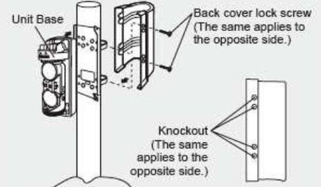
After mounting the units base, fix the back cover on the pole bracket by using the screws (4 pieces). Align the optical axis and check for the operation, then close the cover. (See "3. INSTALLATION")
