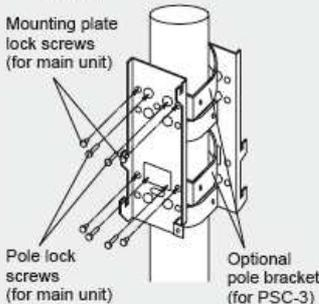
**Note** Do not use pole bracket supplied with the unit
