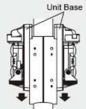
After mounting the units base, align the optical axis and check for the operation, then close the cover. (See "3. INSTALLATION")
