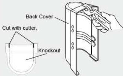
Cut off the knockout portion of the back cover with a cutter, etc.
