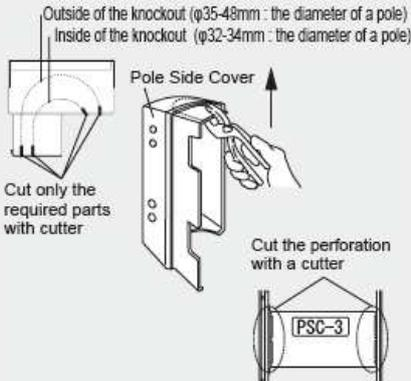
Cut the edge of the knockout (outside or inside) with a nipper and then break the knockout portion with a cutter. Also break the center bridge of the pole side cover along with the perforation.
